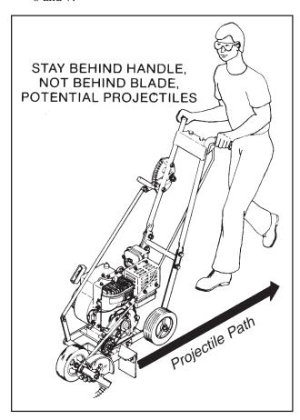
**Figure 1, Proper Operating Position**
